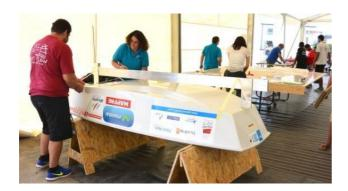
At some events, the Chief Measurer may require full measurement to be carried out on a number of hulls at this station which may include hull shape, materials, positioning of fittings etc.
